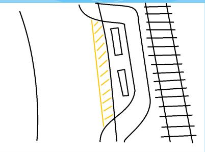
From a PBOT Traffic Engineering Report from Mark Haines (3/25/2014): "[...] Bridge columns narrowed the pavement width by approximately two feet for a length of approximately 70 feet. That width was taken entirely out of the bike lane [...] I recommend referring the request to a CIP list for future consideration."
